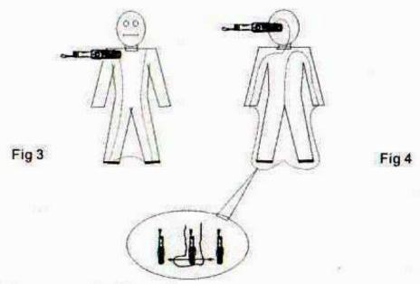
First, to scan the front of the body, pass the detector from the right shoulder down to the ankles and then up to the left shoulder as shown in Figure 3.
