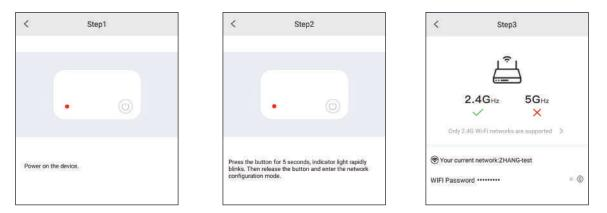
Remarks: Red indicator means status of network; Fast flashing means to enter into network configuration; Slow flashing means network is unusual; Indicator always on means network is ok.
